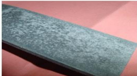
Figure 1 - Aluminum with white hydroxide layer
